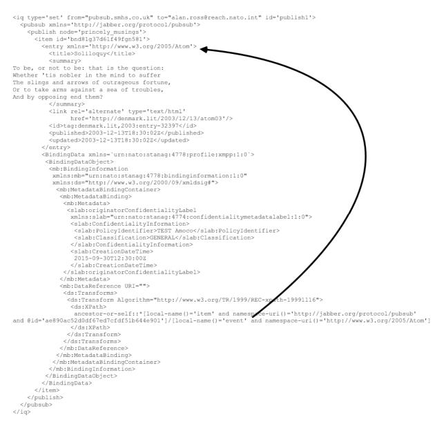
Figure 4-5 Example Detached BDO contained in IQ Stanza
